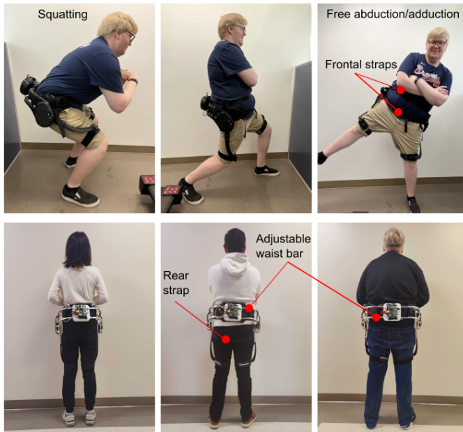
Fig. 2. Our portable hip exoskeleton enables a large range of motion for assisting versatile activities. The width of the back frame can also be extended to provide lateral adjustability to fit people with different waist sizes (one size for all).
